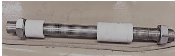
EXAMPLE OF THREADED ROD TOOL USED TO PRESS BEARINGS INTO HOUSING.
